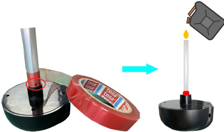
Closing the drain holes, rotating the sensor, and filling the tubes with fuel
